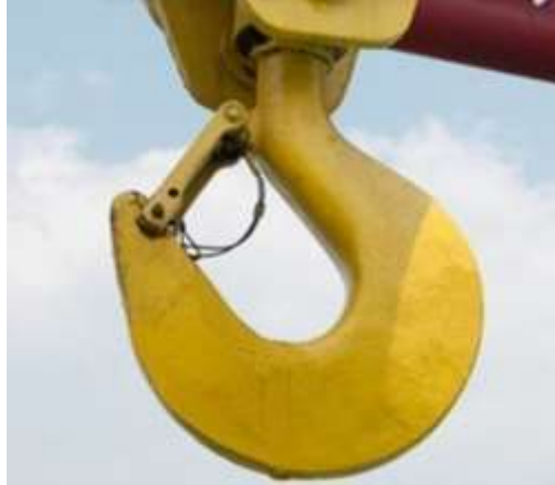
Figure 16 – Crane hook with lockable safety catch
