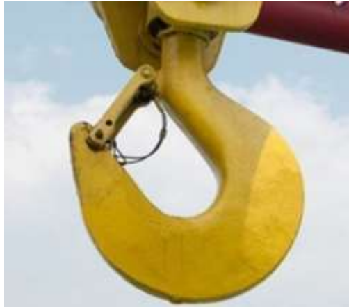
Figure 16 – Crane hook with lockable safety catch
