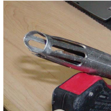
Retro jet showing proximity of nozzle to end of baffle (approx 3 cm)
