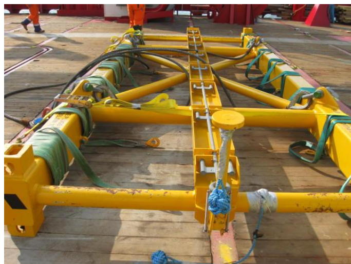
Figure 1 – ROV operable installation frame showing release mechanism
