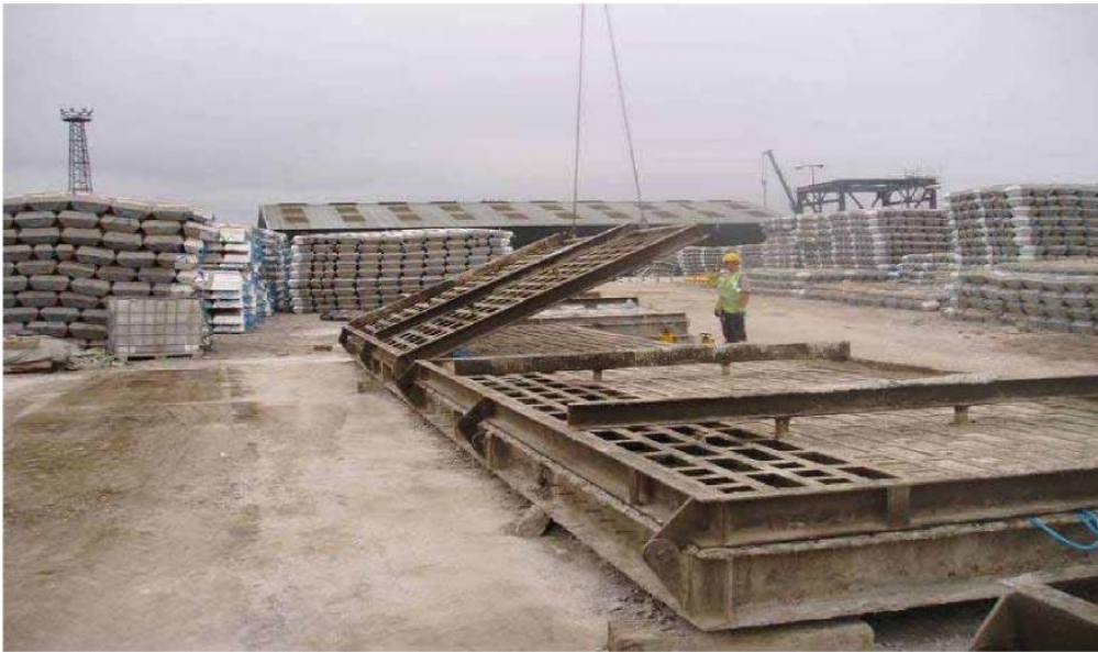
Figure 3 – A well managed manufacturing base is essential for ensuring quality control. Any mattress products that are stored in open sunlight need to be protected from the harmful effects of ultraviolet light
