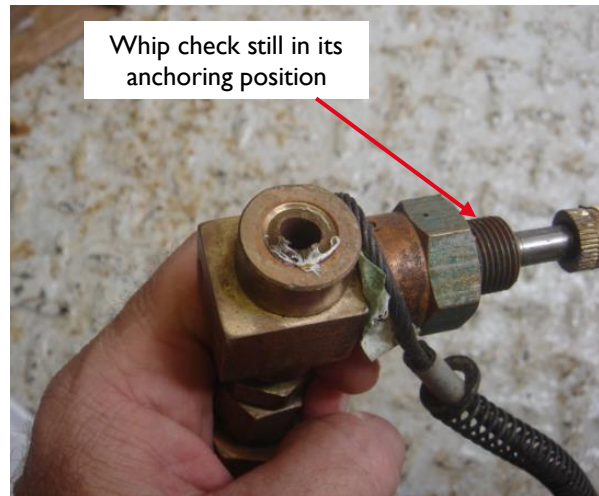
1/4" NPT Nipple snapped off from diver charging manifold
